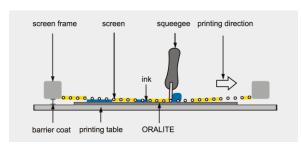
For printing, it is recommend to maintain a medium squeegee speed of approximately 0.75m/s and the squeegee should be applied at an angle of 30° to the print surface.
