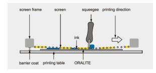
For printing, it is recommend maintaining a medium squeegee speed of approximately 0.75m/s and the squeegee should be applied at an angle of 30° to the print surface.
